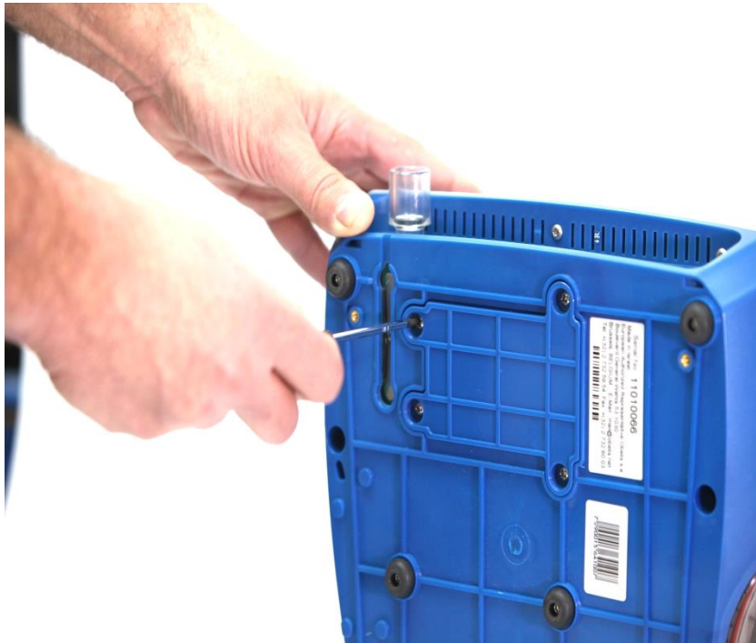
Figure 6 – Removing the Internal Battery Panel
