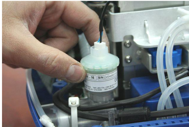
Figure 47 – Removing the Oxygen Sensor
