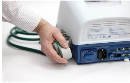
Figure 13 – Air/Oxygen Entrainment Mixer Installation
