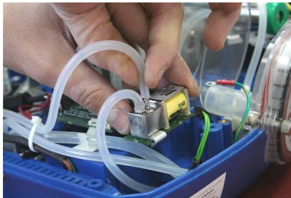
Figure 59 – Removing the Silicon Tubes
