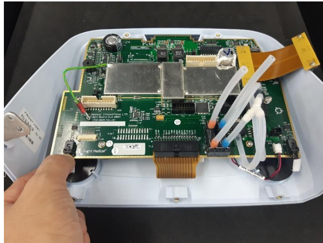
Figure 36 – Disconnecting LS2 connector
