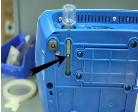
Figure 72 –Adjusting the Pressure Relief Valve
