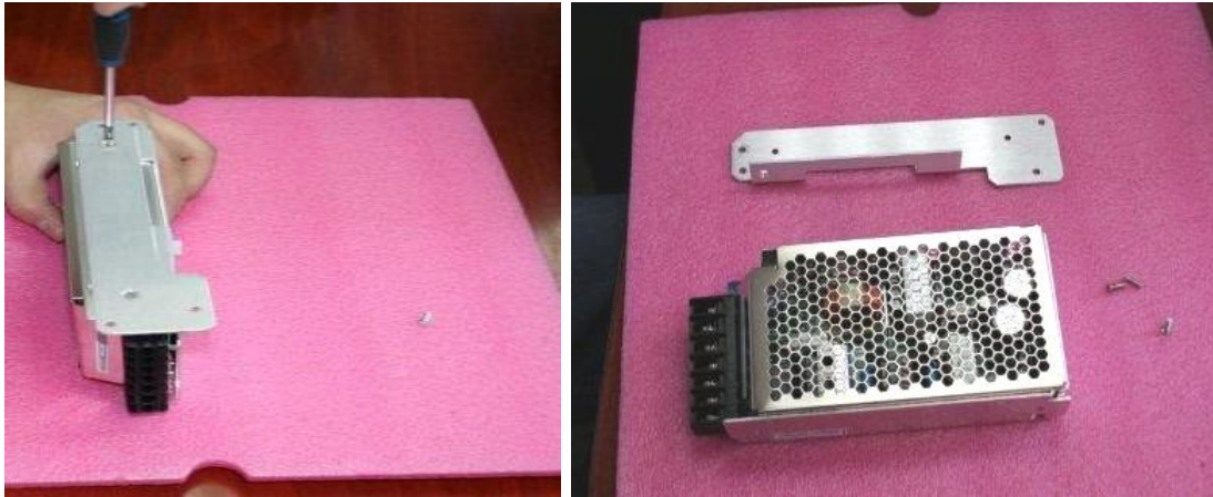
Figure 25 – Detaching the Power Supply from Its Bracket
