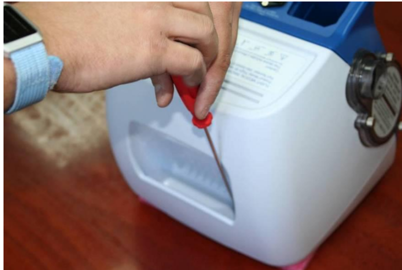
Figure 10 – Removing Screws Inside Handle
