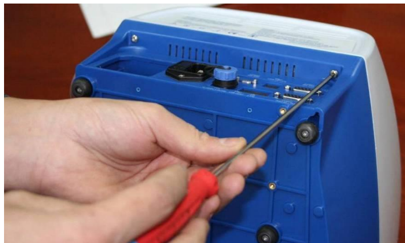
Figure 11 – Removing Back Screws
