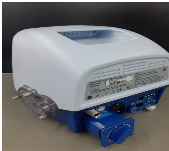
Figure 8 – Removing the Detachable (Main) Battery
