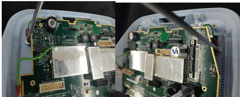
Figure 39 – Detaching the Grounding Screw
