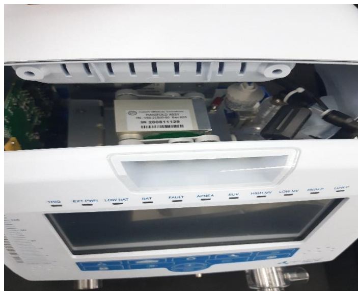
Figure 13 – Removing the Ventilator Cover
