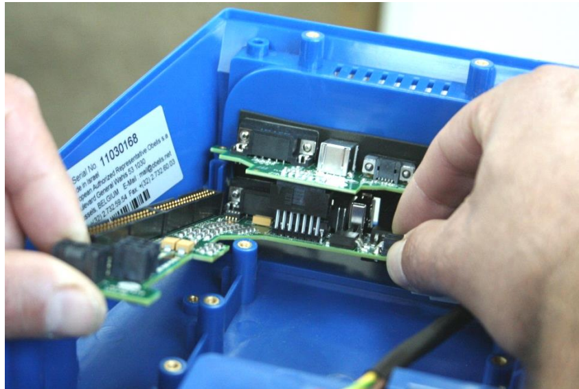
Figure 67 – Removing the Lower Board and D-type Board
