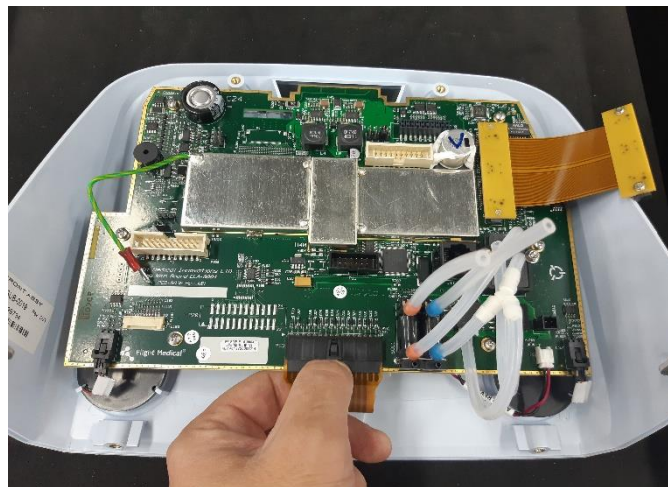
Figure 37 – Disconnecting the P13 Flat Cable
