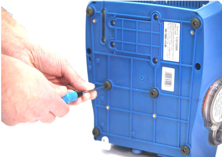
Figure 71 – Removing a Rubber Bumper
