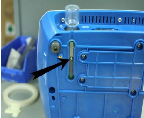
Figure 72 –Adjusting the Pressure Relief Valve
