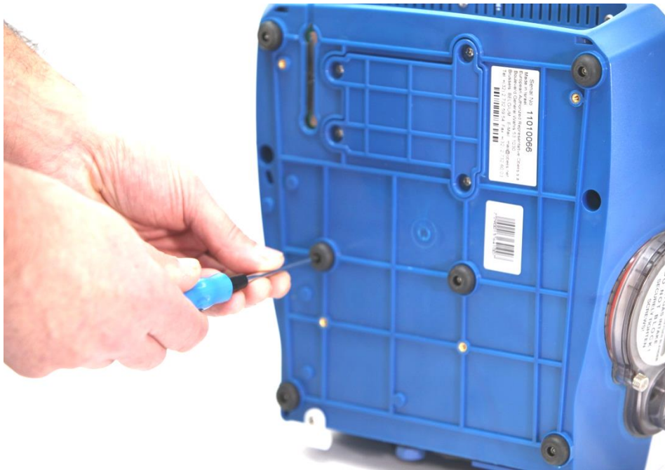
Figure 71 – Removing a Rubber Bumper
