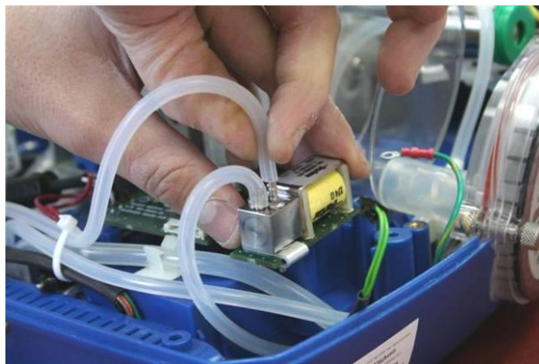
Figure 59 – Removing the Silicon Tubes
