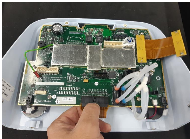
Figure 37 – Disconnecting the P13 Flat Cable
