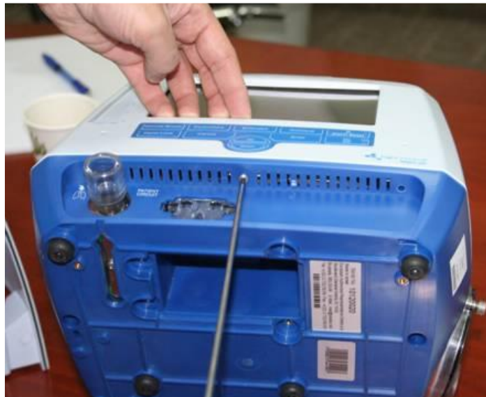
Figure 31 – Loosening the Torx Screws Under the Front Panel
