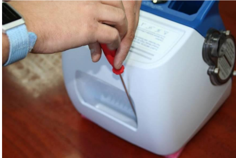
Figure 10 – Removing Screws Inside Handle
