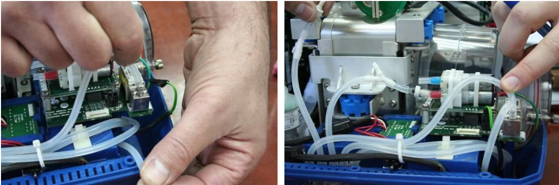
Figure 60 – Connecting the Silicon Tubes
