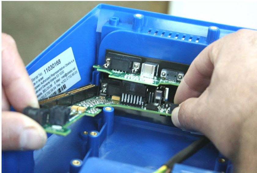
Figure 67 – Removing the Lower Board and D-type Board
