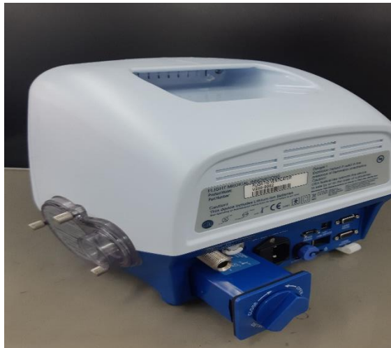
Figure 8 – Removing the Detachable (Main) Battery
