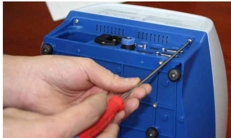
Figure 11 – Removing Back Screws
