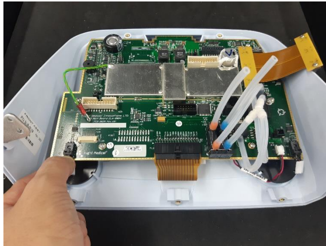
Figure 36 – Disconnecting LS2 connector
