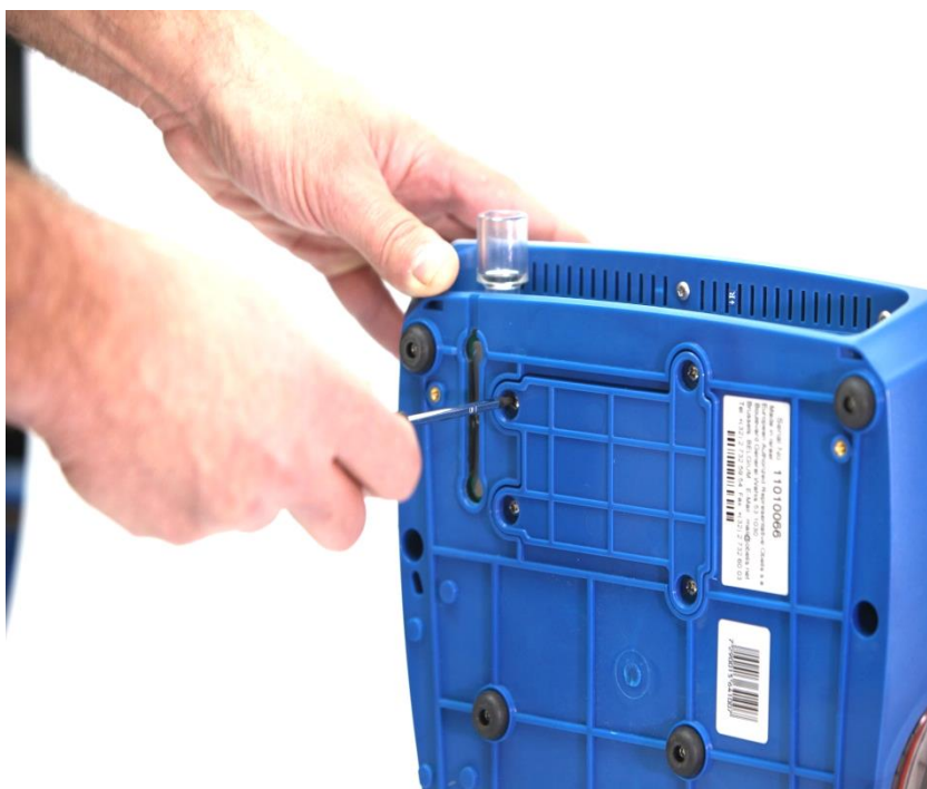
Figure 9 – Removing the Internal Battery Panel
