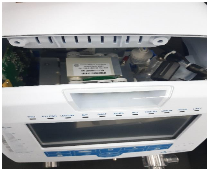
Figure 13 – Removing the Ventilator Cover
