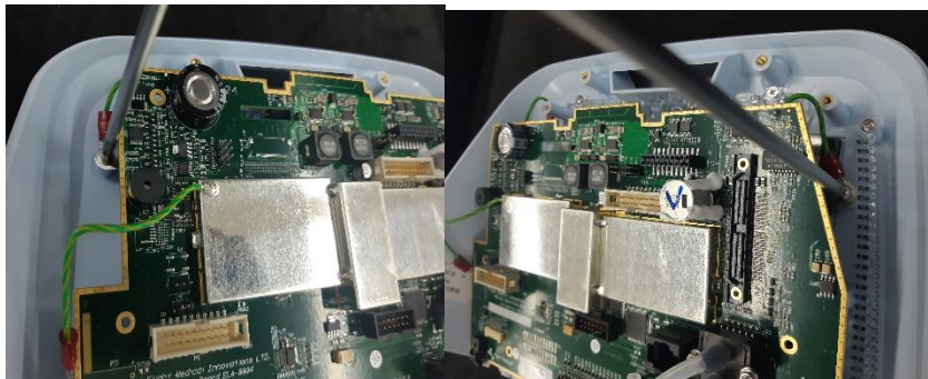
Figure 39 – Detaching the Grounding Screw
