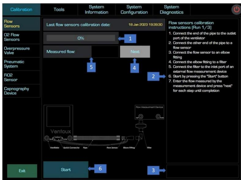
Figure 6-1: Flow Sensors Calibration – Screen Description
