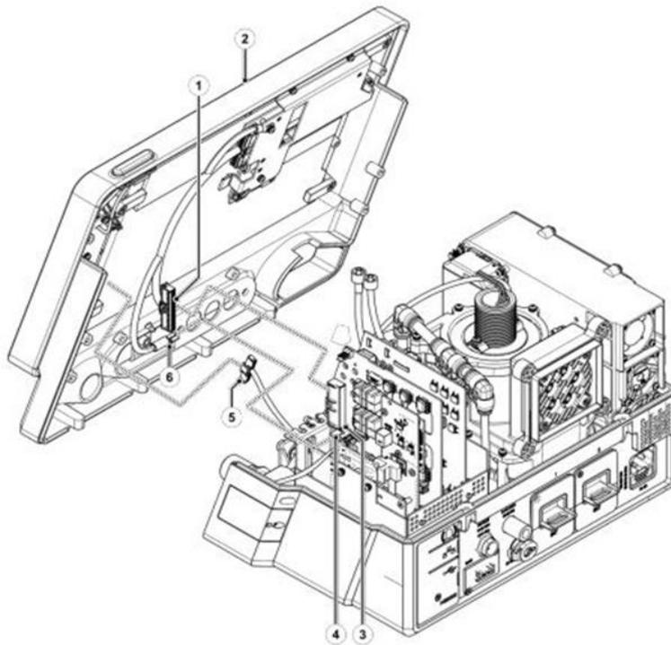
Figure 8-4: 12" Front Removal (3 of 3)
