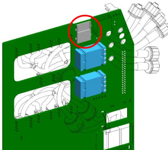
*Figure 12-1: SD Card Slot in Main Board*
