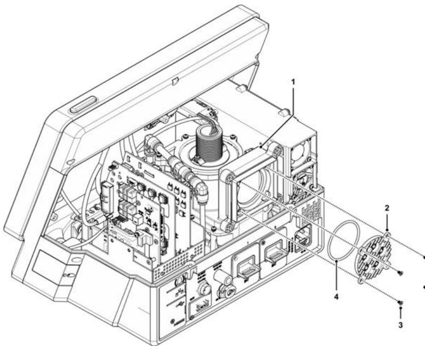
Figure 8-34: Blower One Way Valve Cassette Replacement
