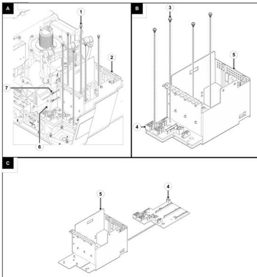
Figure 8-40: Base Board Assy – Removal and Installation
