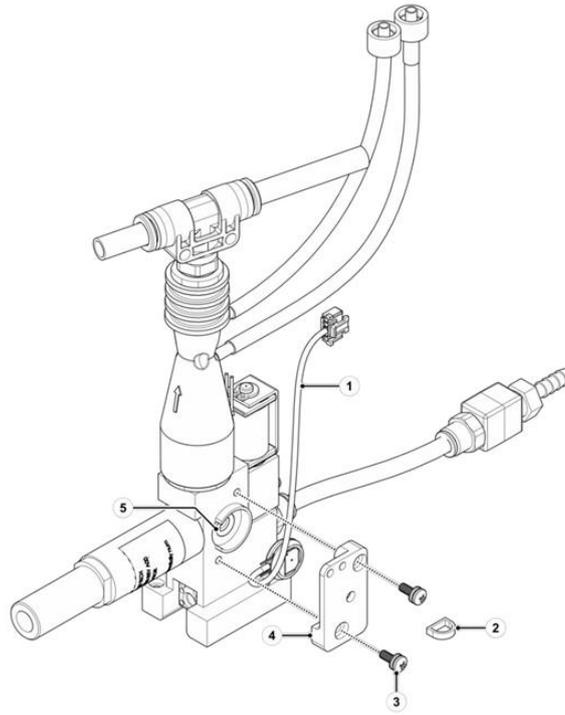
Figure 8-25: O2 Pressure Sensor Replacement
