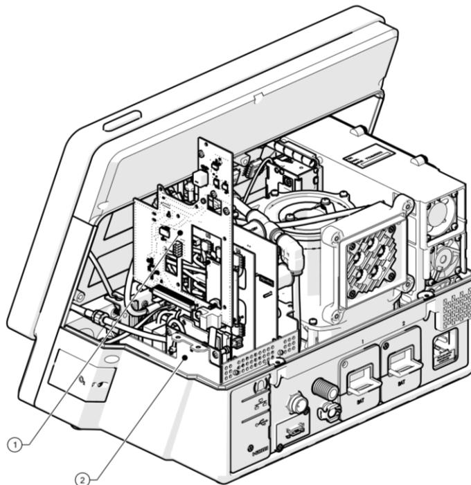
Figure 8-10: Extended Board Assy Replacement
