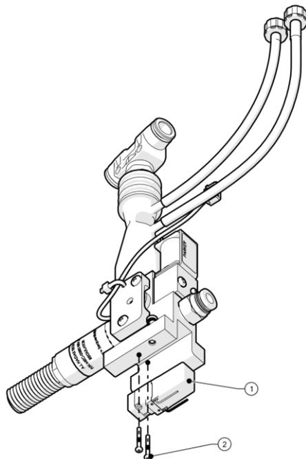
Figure 8-22: Valve Nebulizer Replacement
