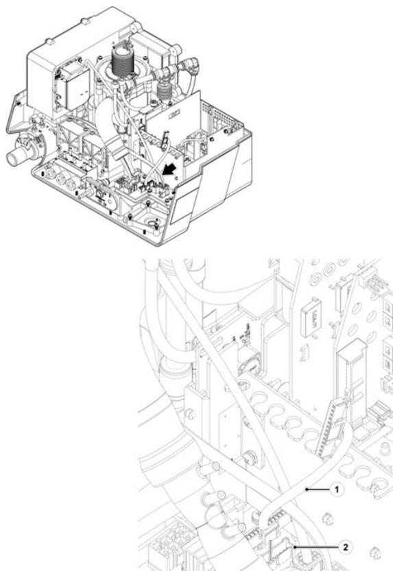
Figure 8-45: Base Board - Front Panel Cable Replacement
