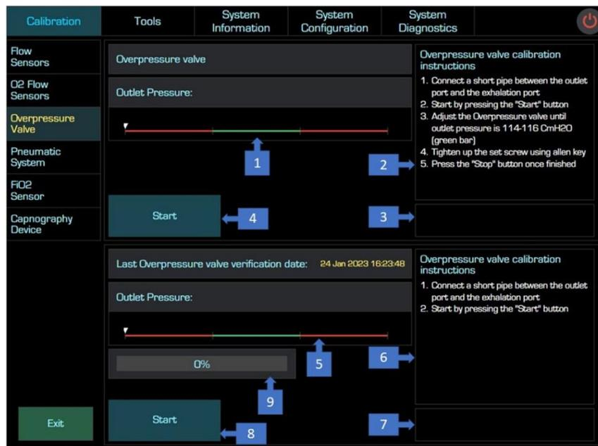
Figure 6-3: Overpressure Value Calibration - Screen Description
