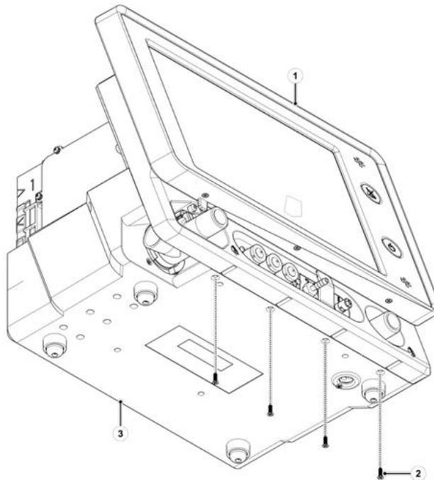
Figure 8-6: 12" Front Installation (2 of 3)
