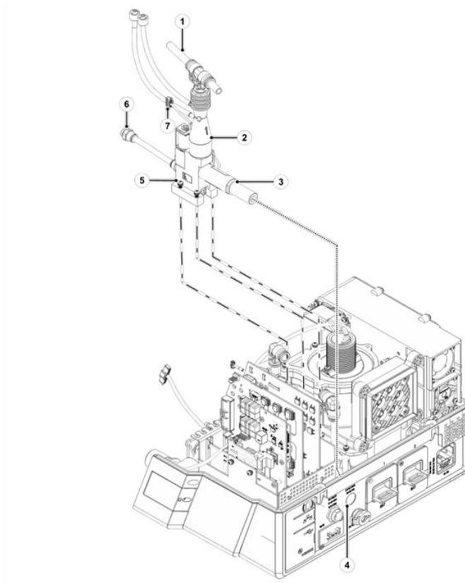
Figure 8-21: Internal Mixer Replacement (3 of 3)
