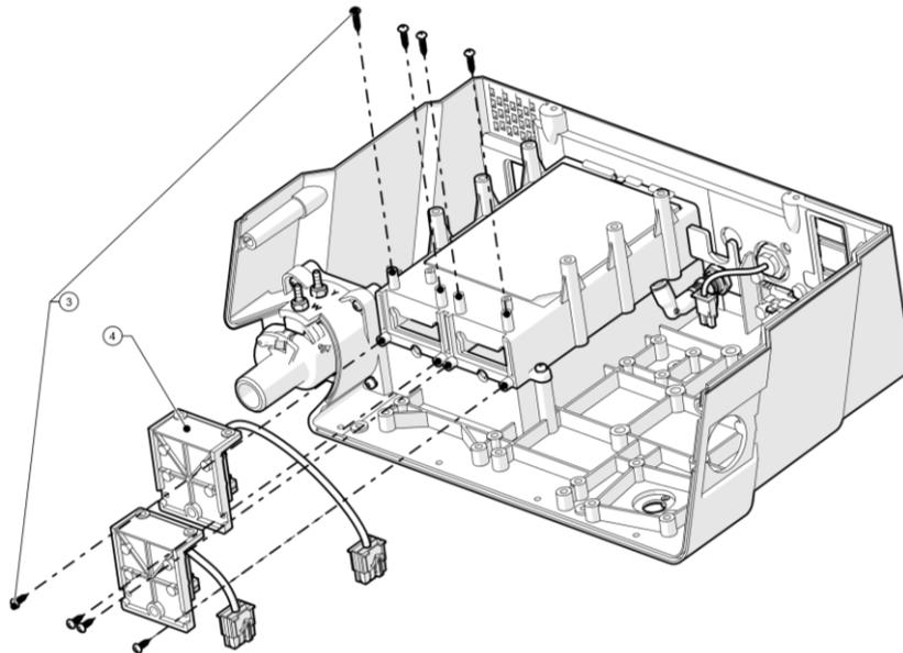
Figure 8-54: Batteries – Base Board Cable Assy Replacement (2 of 3)
