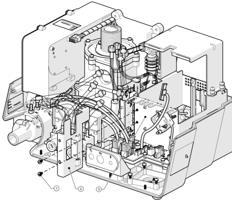
Figure 8-20: Internal Mixer Replacement (2 of 3)
