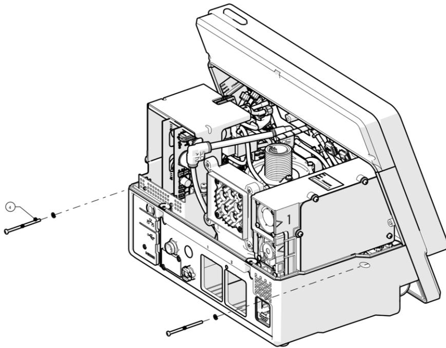
Figure 8-3: 12" Front Removal (2 of 3)
