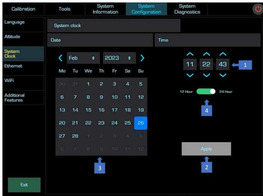
*Figure 6-18: System Clock Setup – Screen Description*
