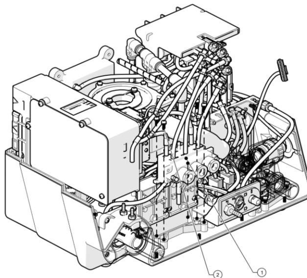
Figure 8-33: Three Way Valve Replacement
