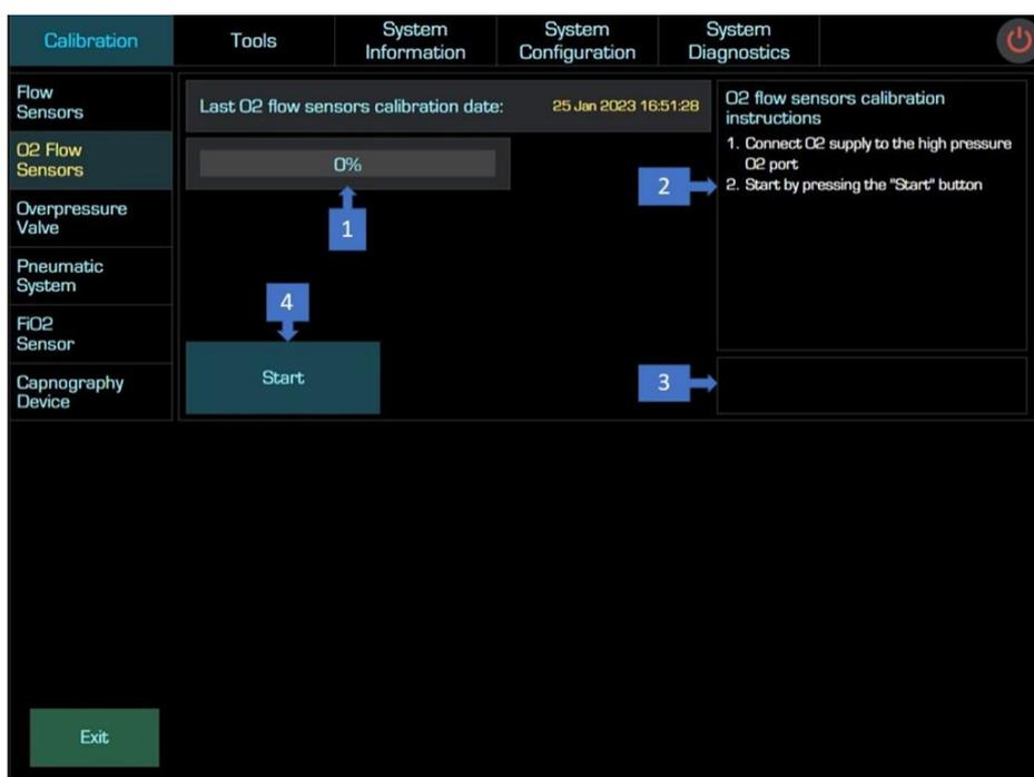
Figure 6-2: O2 Flow Sensors Calibration – Screen Description
