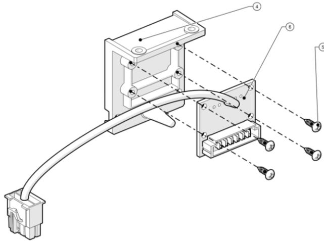
Figure 8-55: Batteries – Base Board Cable Assy Replacement (3 of 3)
