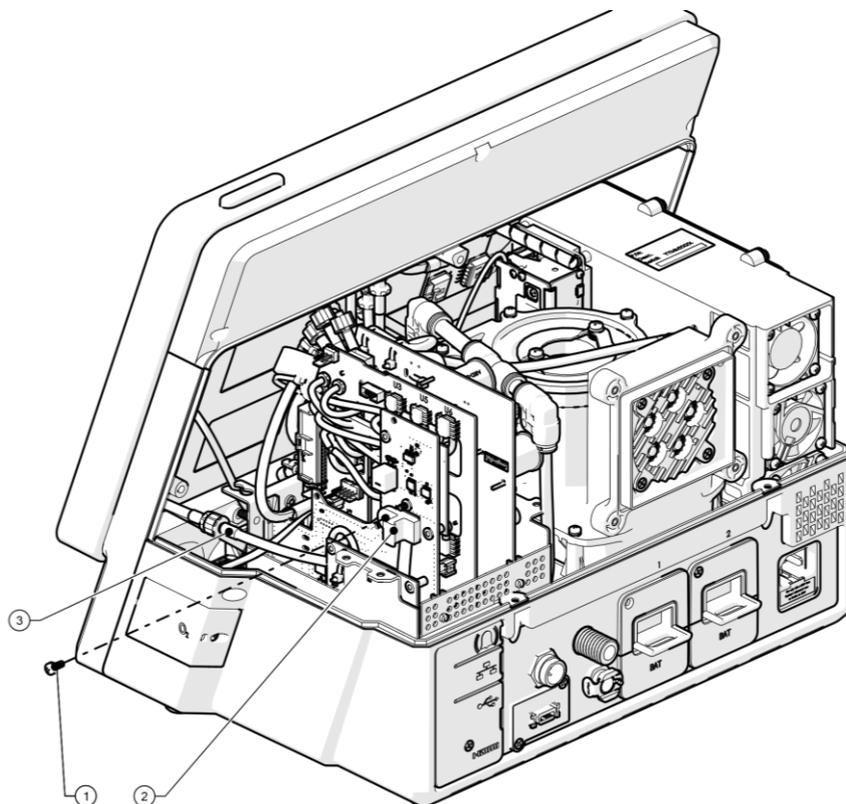
Figure 8-11: Nellcor SpO2 PCBA Replacement (1 of 2)
