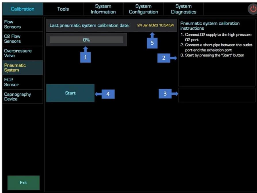
Figure 6-4: Pneumatic System Calibration – Screen Description
