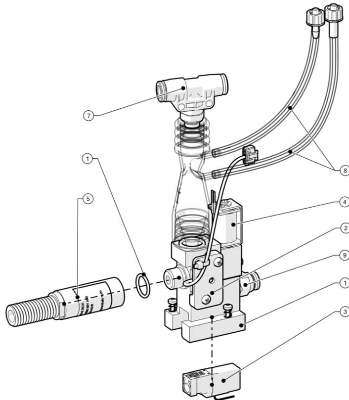
Figure 8-52: First Assembly Stage of O2 Mixer Replacement
