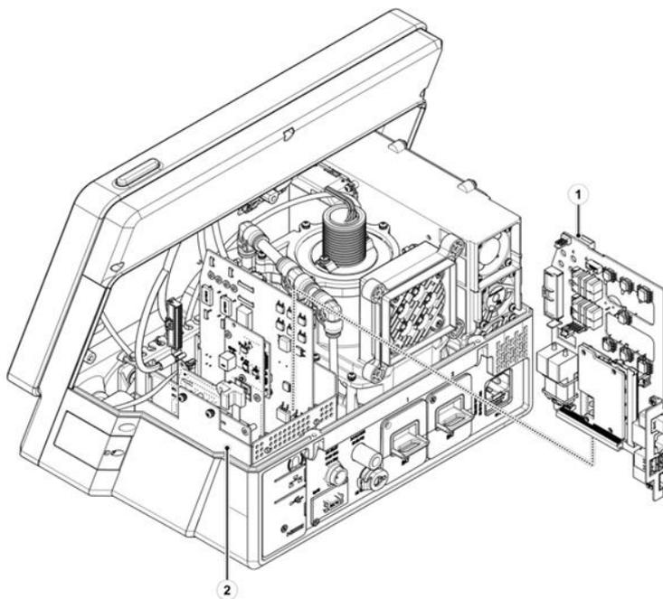
Figure 8-13: Main board Assy. Replacement
