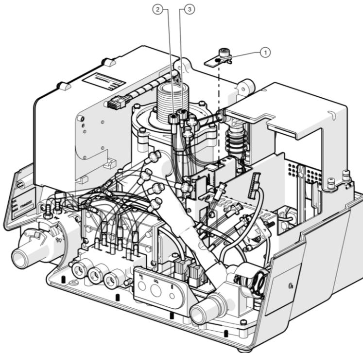
Figure 8-19: Internal Mixer Replacement (1 of 3)
