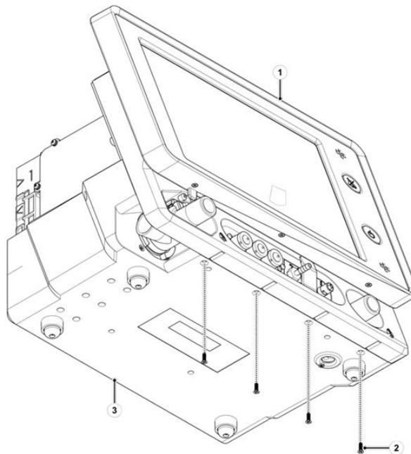
Figure 8-2: 12" Front Removal (1 of 3)
