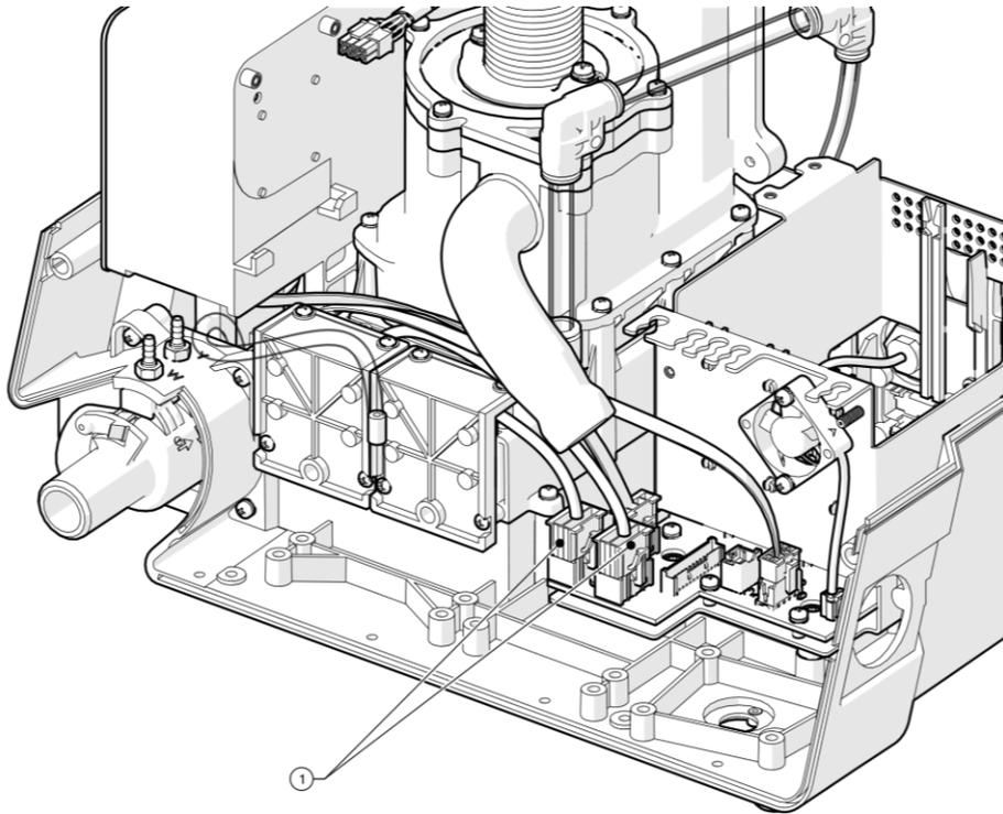
Figure 8-53: Batteries – Base Board Cable Assy Replacement (1 of 3)
