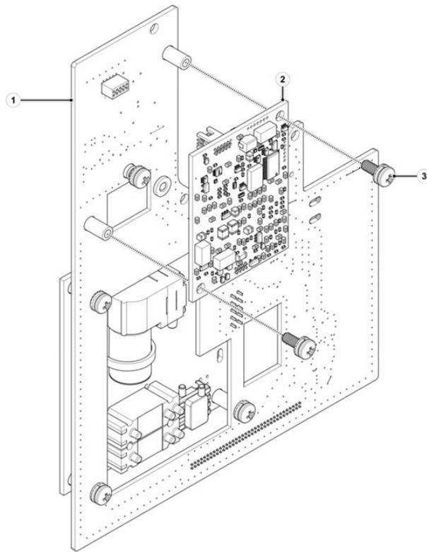
Figure 8-12: Nellcor SPO2 PCBA Replacement (2 of 2)
