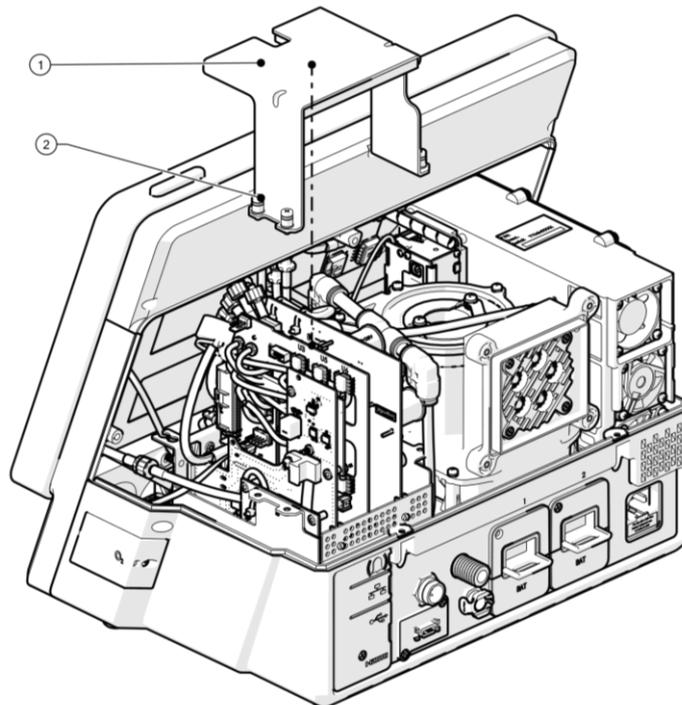
Figure 8-8: PCB Cage Cover Removal and Installation
