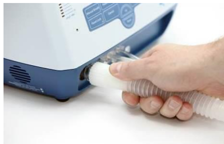
Figure 9 – Patient Circuit (22 mm Tube)
