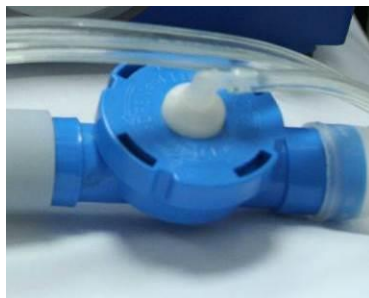
Figure 33 – Exhalation Valve Assembly
