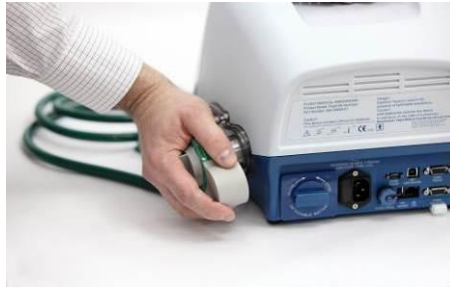
Figure 13 – Air/Oxygen Entrainment Mixer Installation
