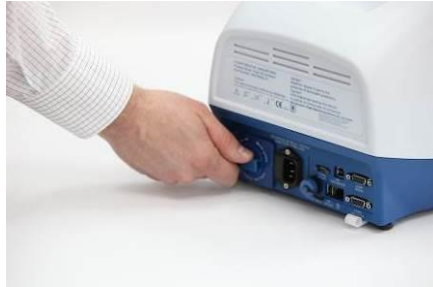
Figure 6 – Installing the Detachable Battery
