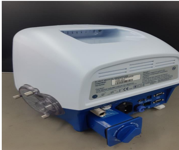
Figure 6 – Removing the Detachable (Main) Battery
