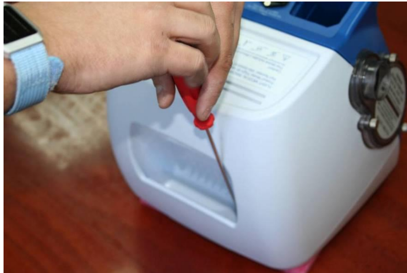
Figure 8 – Removing Screws Inside Handle
