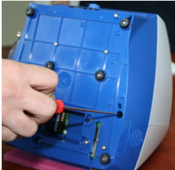
Figure 10 – Removing the Bottom Panel Screws
