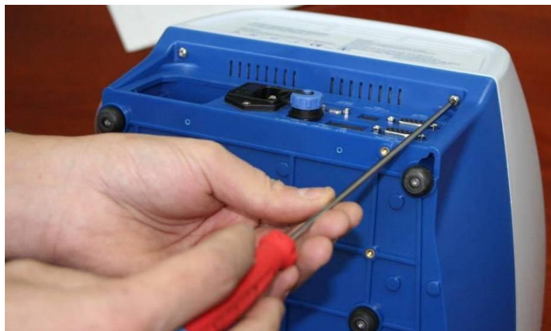
Figure 9 – Removing Back Screws
