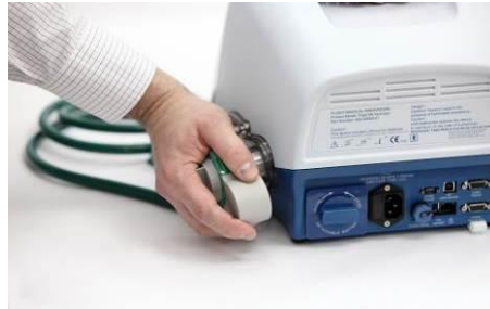
Figure 10 – Air/Oxygen Entrainment Mixer Installation
