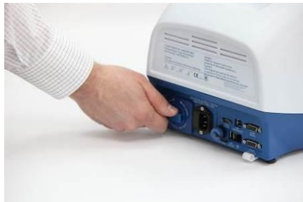
Figure 6 – Installing the Detachable Battery
