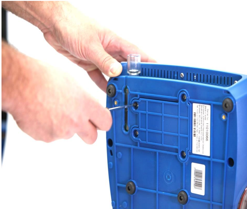
Figure 7 – Removing the Internal Battery Panel
