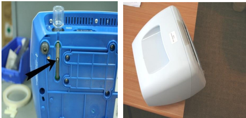
Figure 42 – Adjusting the Pressure Relief Valve
