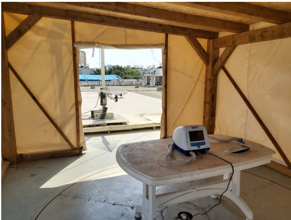
Photo of test setup for Radiated Disturbance Above 200 MHz
