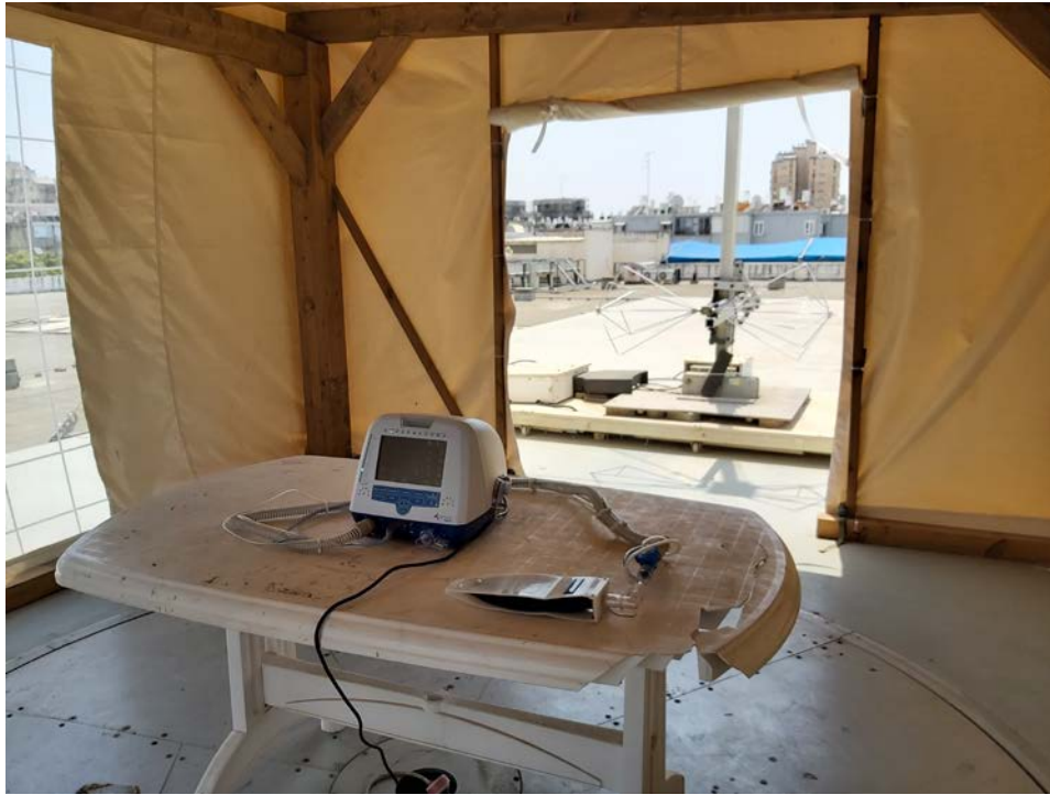
Photo of test setup for Radiated Disturbance Below 200 MHz
