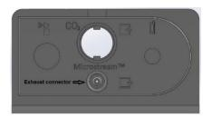
Microstream capnography connector and exhaust connector
