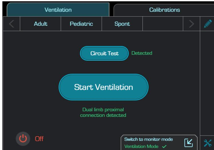
The result of the circuit test and the circuit type detected is shown on the screen. If the circuit test fails, the "Start Ventilation" button is disabled.
