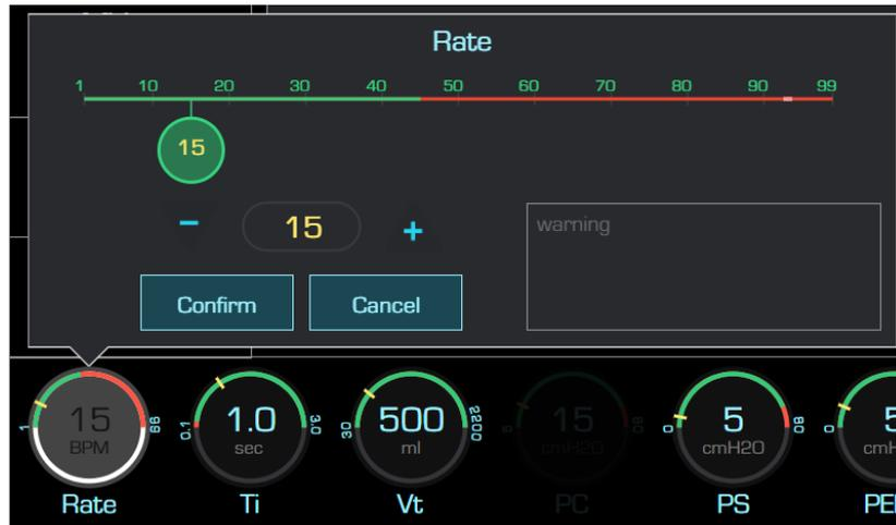
2. Adjust the numeric value using the +/- in the displayed bar or by dragging the value indicator over the displayed bar.
