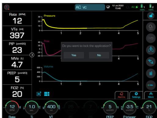
Once tapping "Yes" the screen is locked. When trying to tap the screen the lock symbol will appear:
