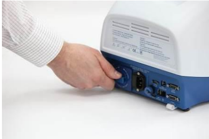
Figure 6 – Installing the Detachable Battery
