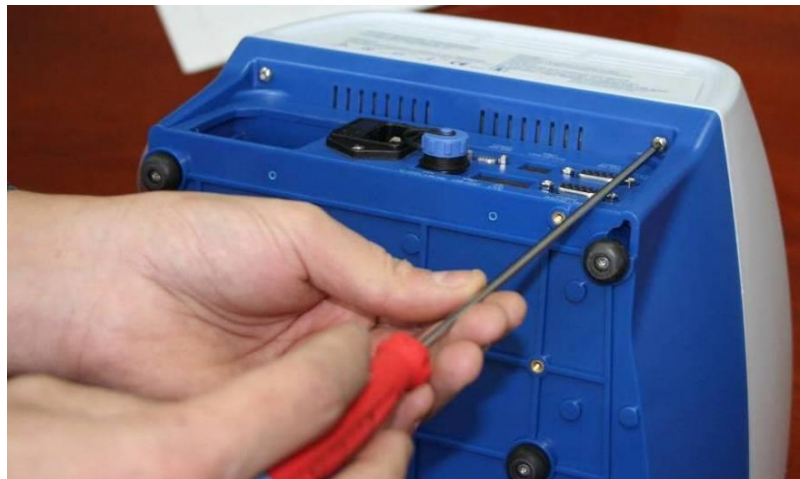
Figure 9 – Removing Back Screws
