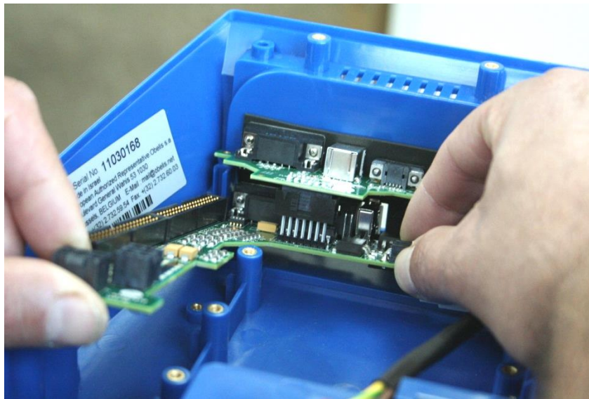
Figure 39 – Removing the Lower Board and D-type Board
