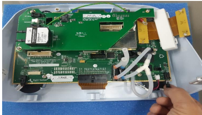
Figure 26 – Disconnecting LS2 connector
