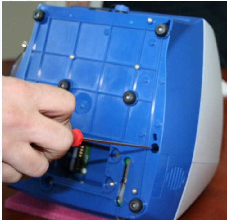
Figure 10 – Removing the Bottom Panel Screws
