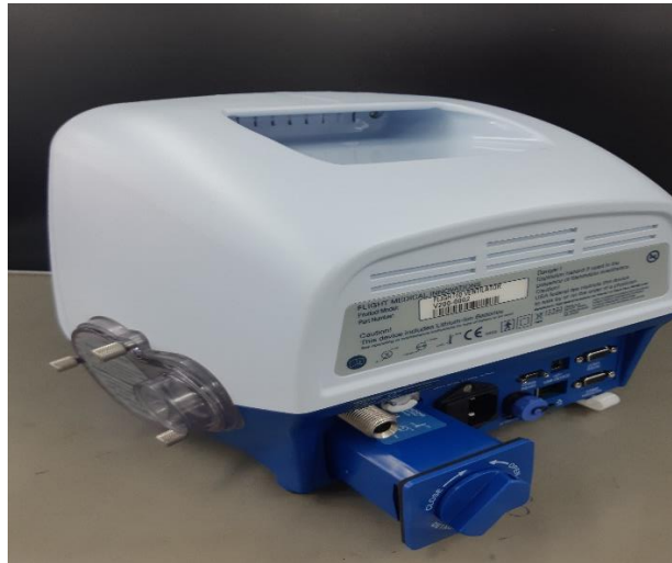
Figure 6 – Removing the Detachable (Main) Battery
