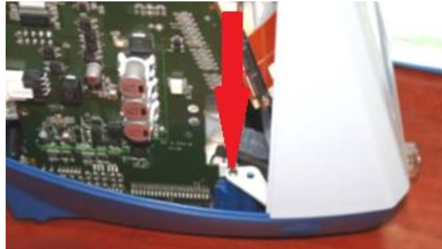
Figure 22 – Torx Screws on Front Panel Bracket
