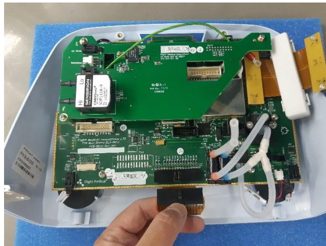
Figure 27 – Disconnecting the P13 Flat Cable
