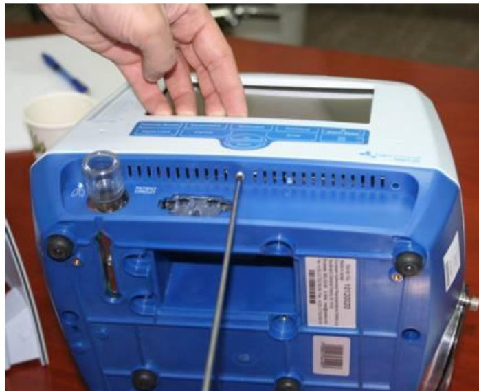
Figure 21 – Loosening the Torx Screws Under the Front Panel
