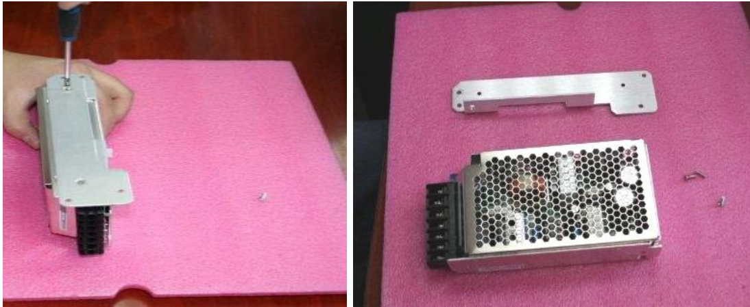
Figure 25 – Detaching the Power Supply from Its Bracket
